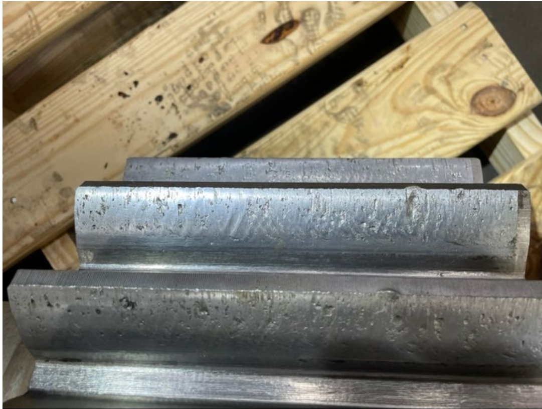
Pitting on south pinion gear
