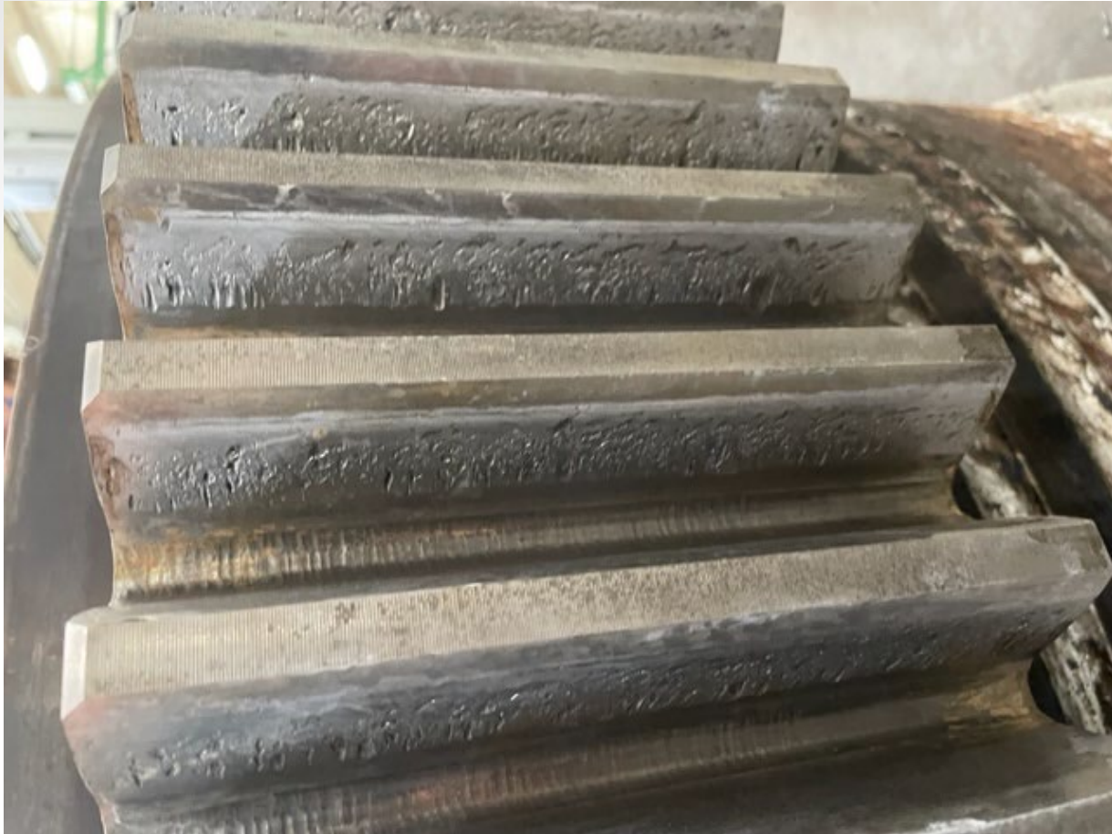
Pitted north drum gear
